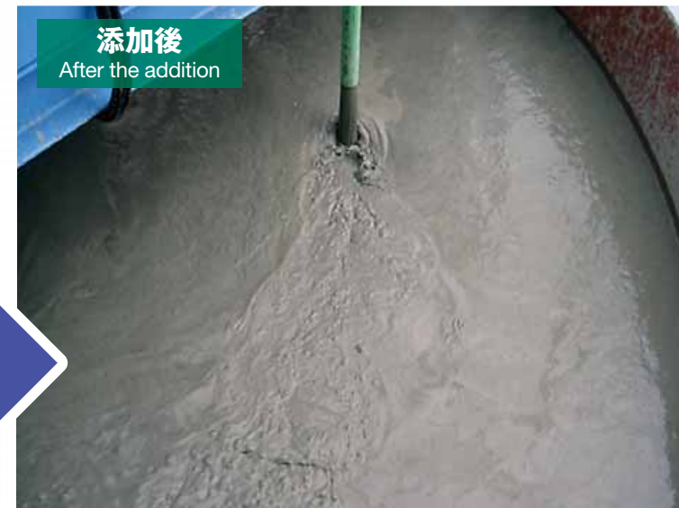
気泡シールド工法の掘削土流体輸送での FT-01 消泡効果(調整槽) Defoaming effect of FT-01 in the Regulation Tank for Hydraulic Transport System
